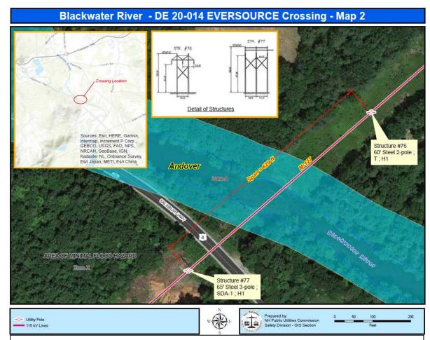
**Figure 1:** 115kV line, designated as the M127 Transmission Line, is a span of approximately 629 feet between structures # 76 and # 77, across the Blackwater River in the Town of Andover, NH.
