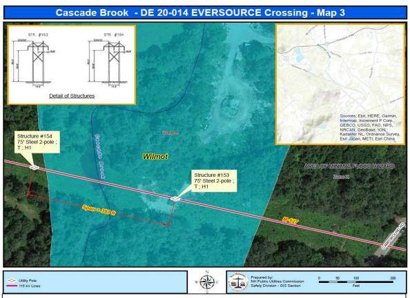
**Figure 1:** 115kV line, designated as the M127 Transmission Line, is a span of approximately 393 feet between structures # 153 and # 154, across the Cascade Brook in the Town of Wilmot, NH.
