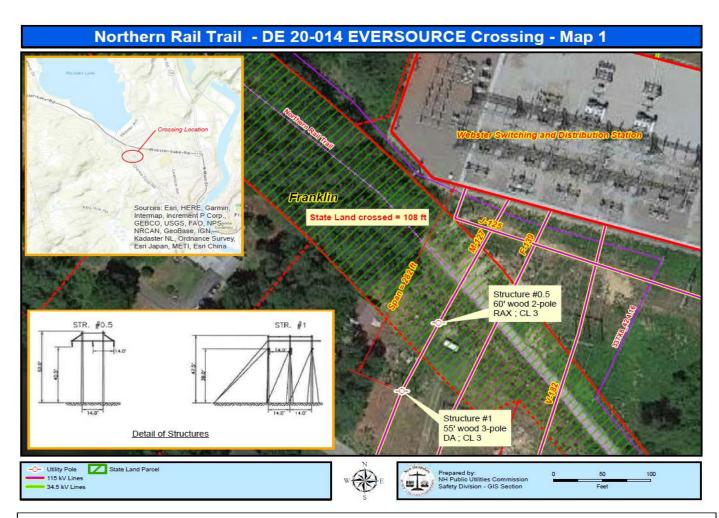
**Figure 1:** 115kV line, designated as the M127 Transmission Line, is a span of approximately 282 feet between Webster Substation and Structure # 1, with a span of approximately 108 ft. crossing State Land in the Town of Franklin, NH. State owned land is shown above as green hash marks
