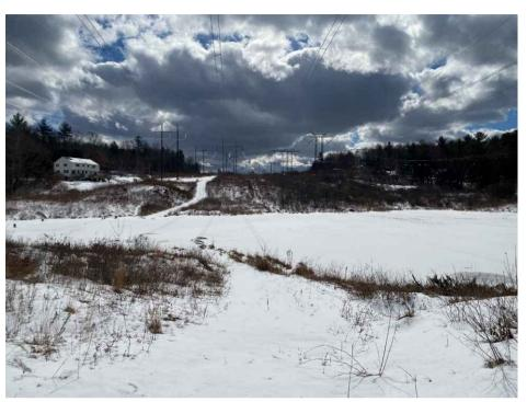
Photograph No. 1: Looking northwesterly at proposed access across Wetland HW-5.1 towards Structure 80 of the 326 Line to be replaced. Timber matting will be used in the wetland portion of the access route.
