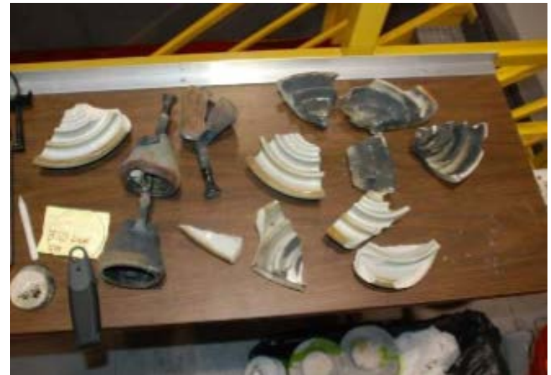
Fragments of Failed PINCO Insulator – Line 310
