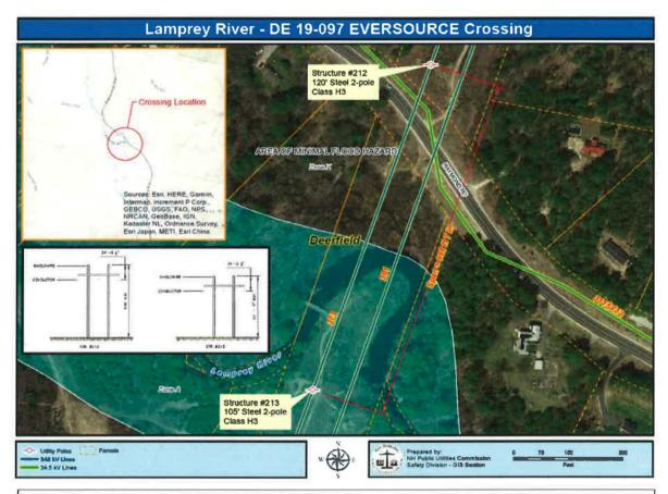
**Figure 1:** 345kV line, designated as the 373 Line, is a span of approximately 996.7 feet between structures # 212 and #213, across the Lamprey River in Deerfield, NH.
