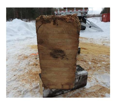
Rotting Cross Section – R187 Line, Structure #7
