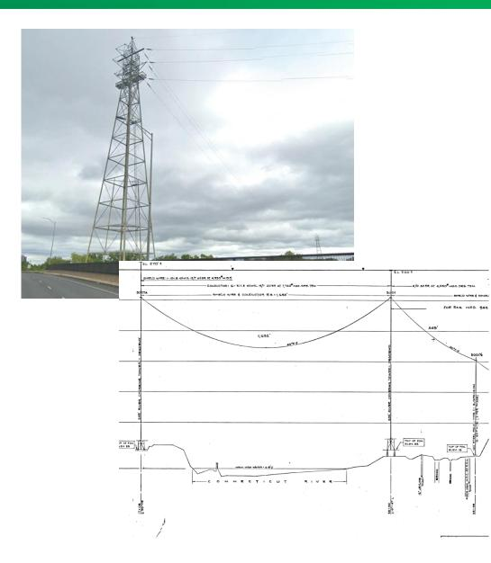
On long spans, ACCR, ACCC and TS conductors offer the ability for increased tensions to have lower sag and therefore short structures
