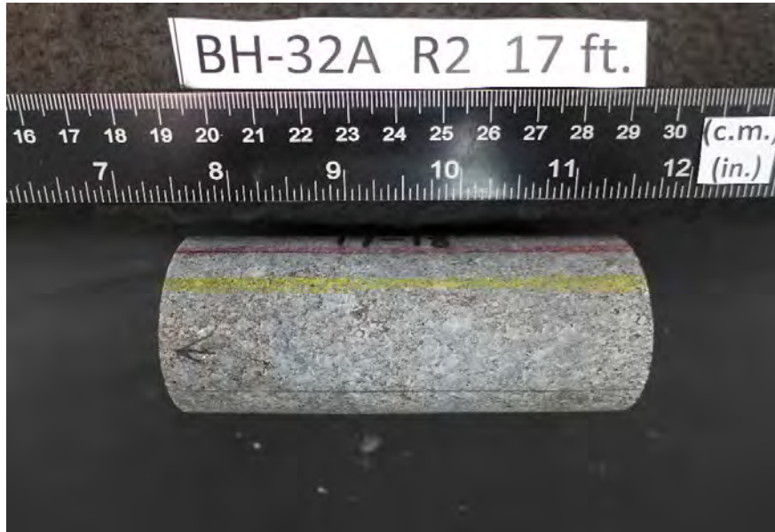
After cutting and grinding
