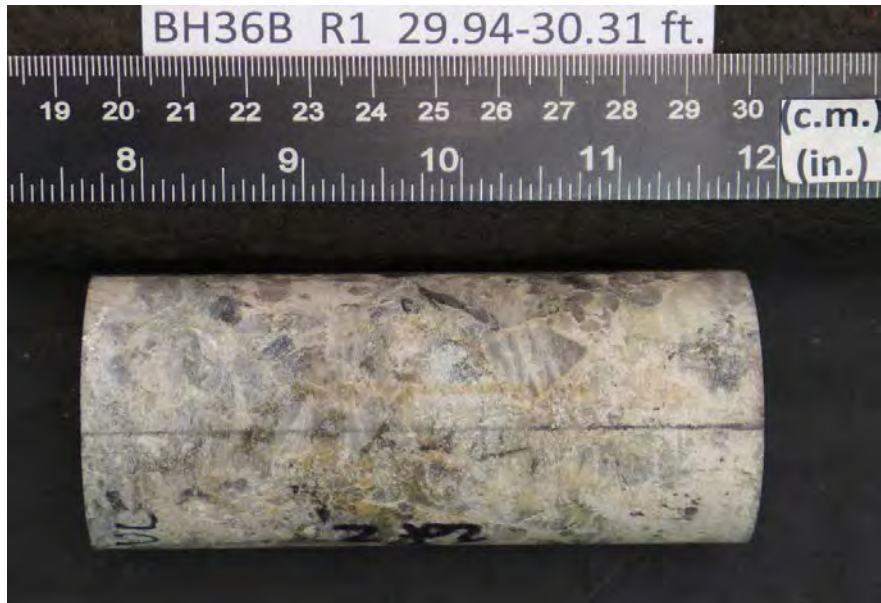
After cutting and grinding
