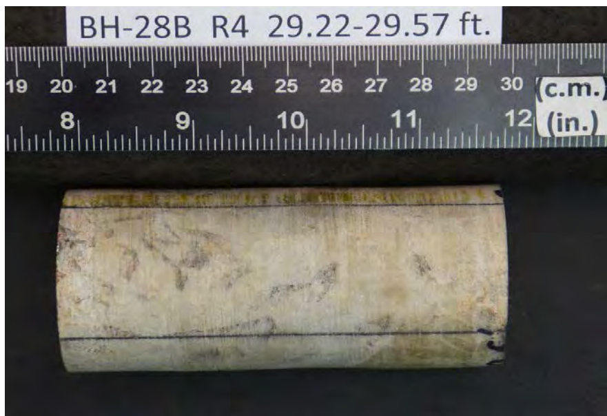
After cutting and grinding
