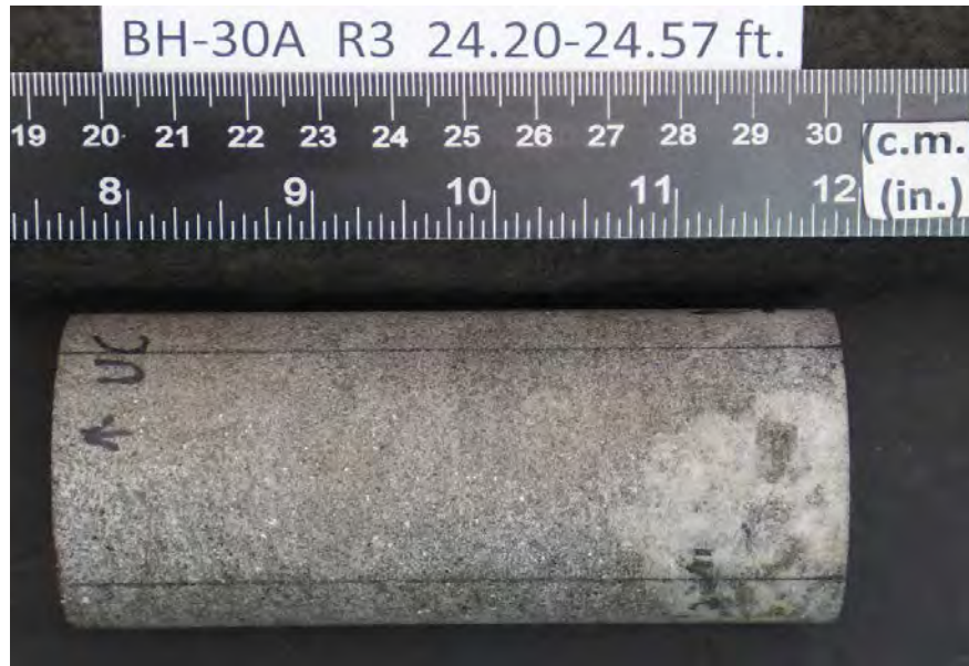
After cutting and grinding
