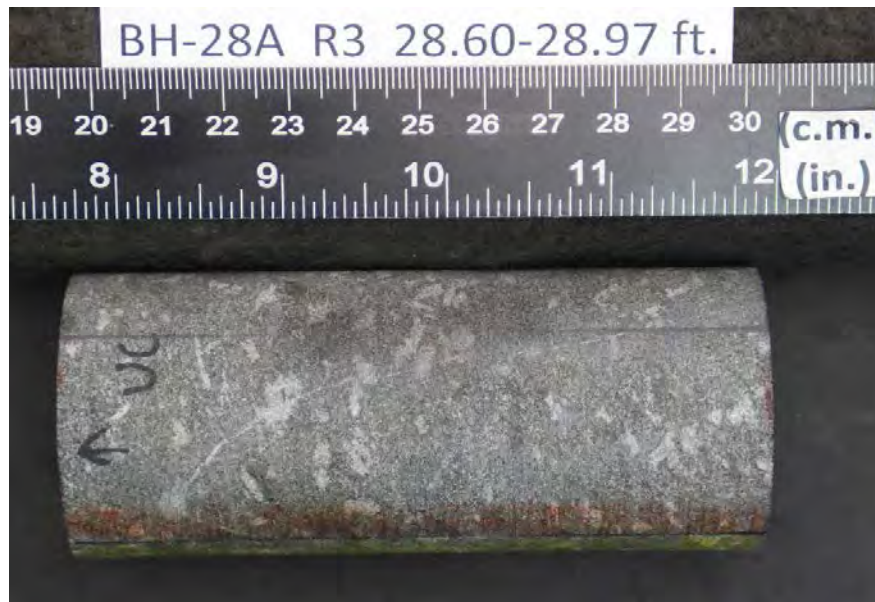
After cutting and grinding
