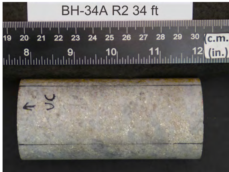
After cutting and grinding
