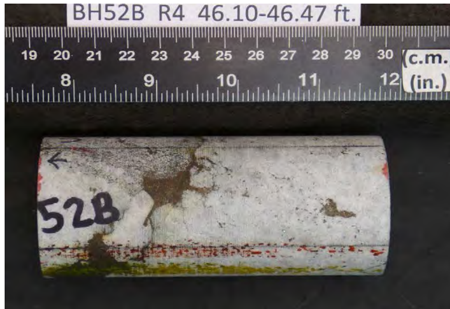
After cutting and grinding
