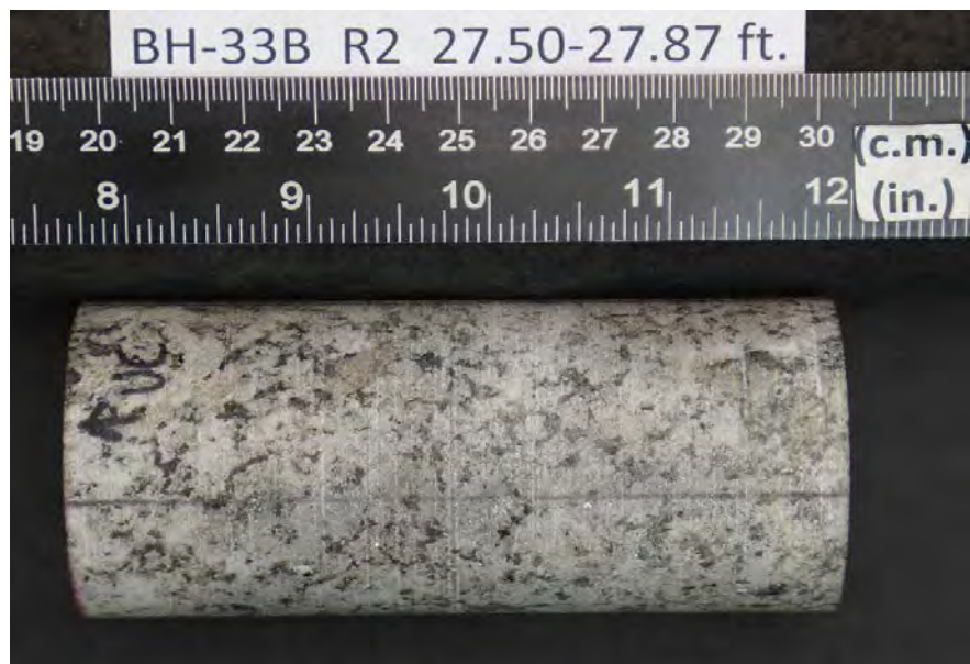
After cutting and grinding
