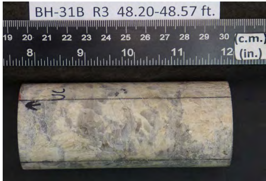
After cutting and grinding
