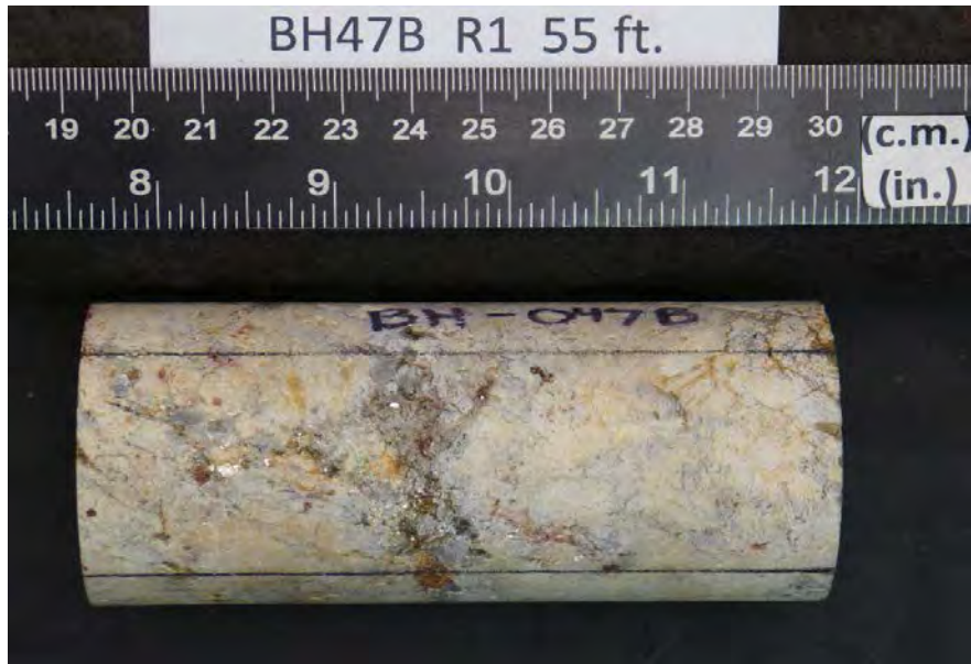
After cutting and grinding
