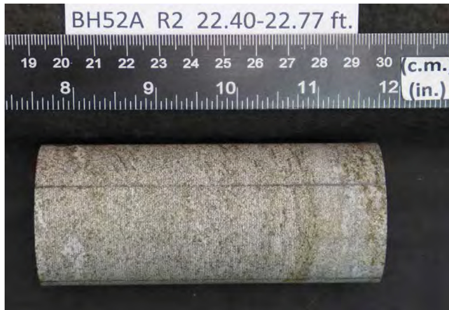
After cutting and grinding
