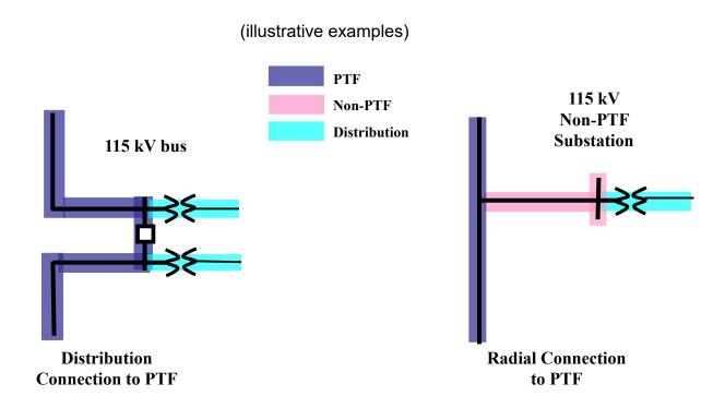
Eversource has distribution connections and radial transmission connections.
