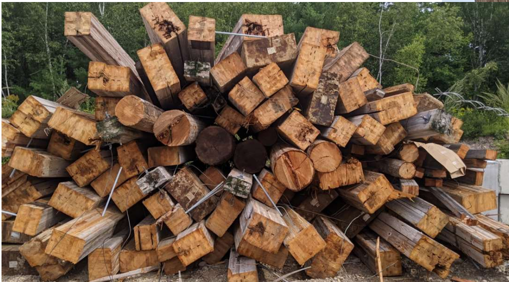
Left: G128 Line – Highly Degraded Laminated Wood Structures with Cracks, Internal Rot, and Insect Damage
