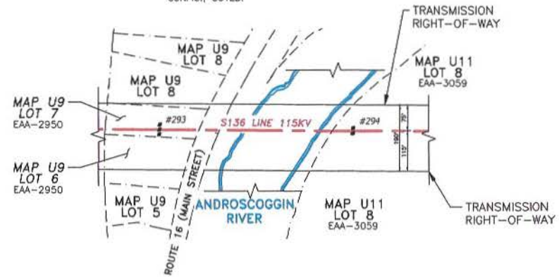
STR 294: IS A SINGLE CIRCUIT STEEL DEADEND STRUCTURE, HORIZONTAL CONFIG., GUYED.
